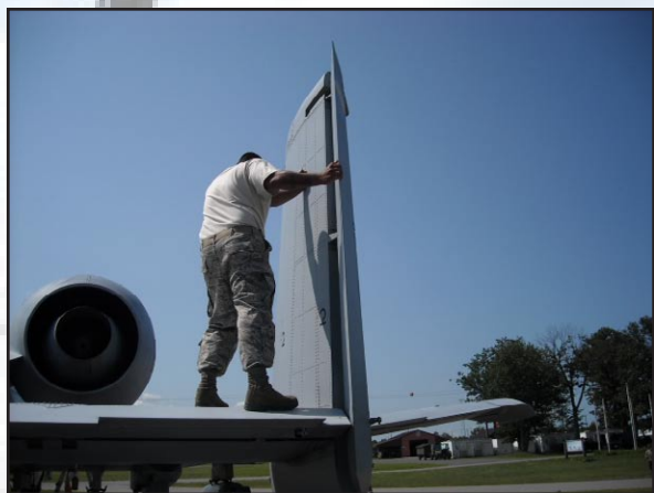
Master Sgt. Tony Thalachira, a crew chief from the 111th Aircraft Maintenance Squadron, performs a post-flight check on the rudder of an A-10 Thunderbolt.
