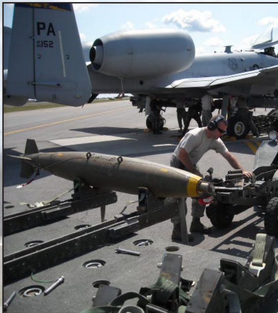
Tech. Sgt. Dennis Donahue preps a live MK-82 low drag bomb before it is lifted and attached to the aircraft, during live loading operations at Fort Drum.
