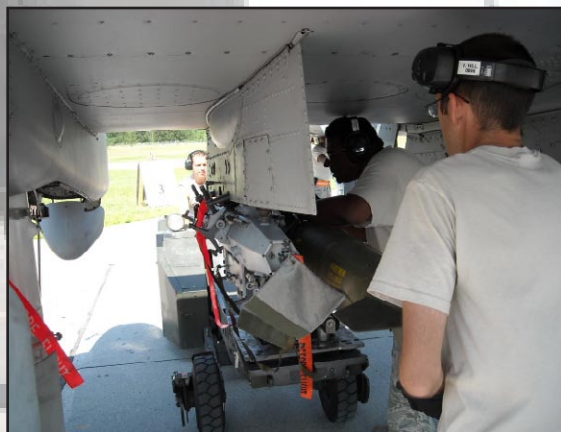
Tech Sgt. Vance Sample (right) locks in a MK-82 on a Triple Ejector Rack (TER), while other members of the crew assist. The three-man team includes Staff Sgt. Ryan Somers and Airman 1st Class Vince Hill.
