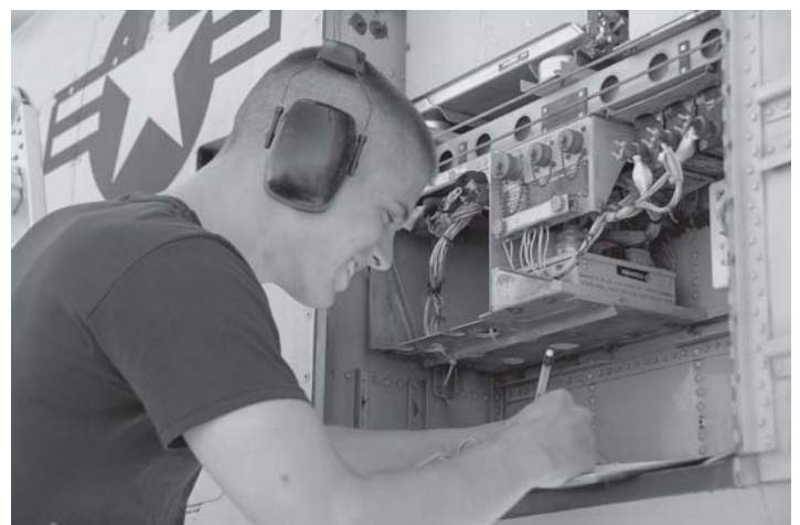
SrA Vincent Franchino, 111th Maintenance, inspects the accelerometer readings which measures g-loads on the air frame. (Photo by SSgt. Marie Harmon).
